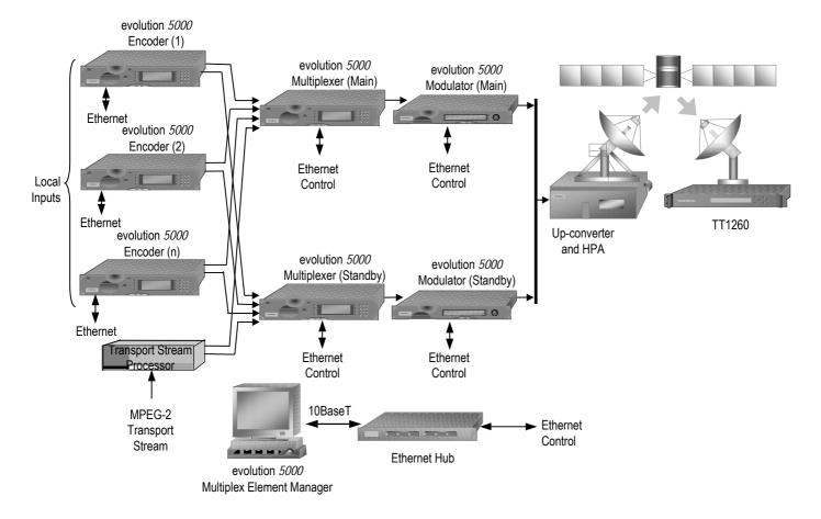
Figure 1.3: Typical Satellite Compression System
